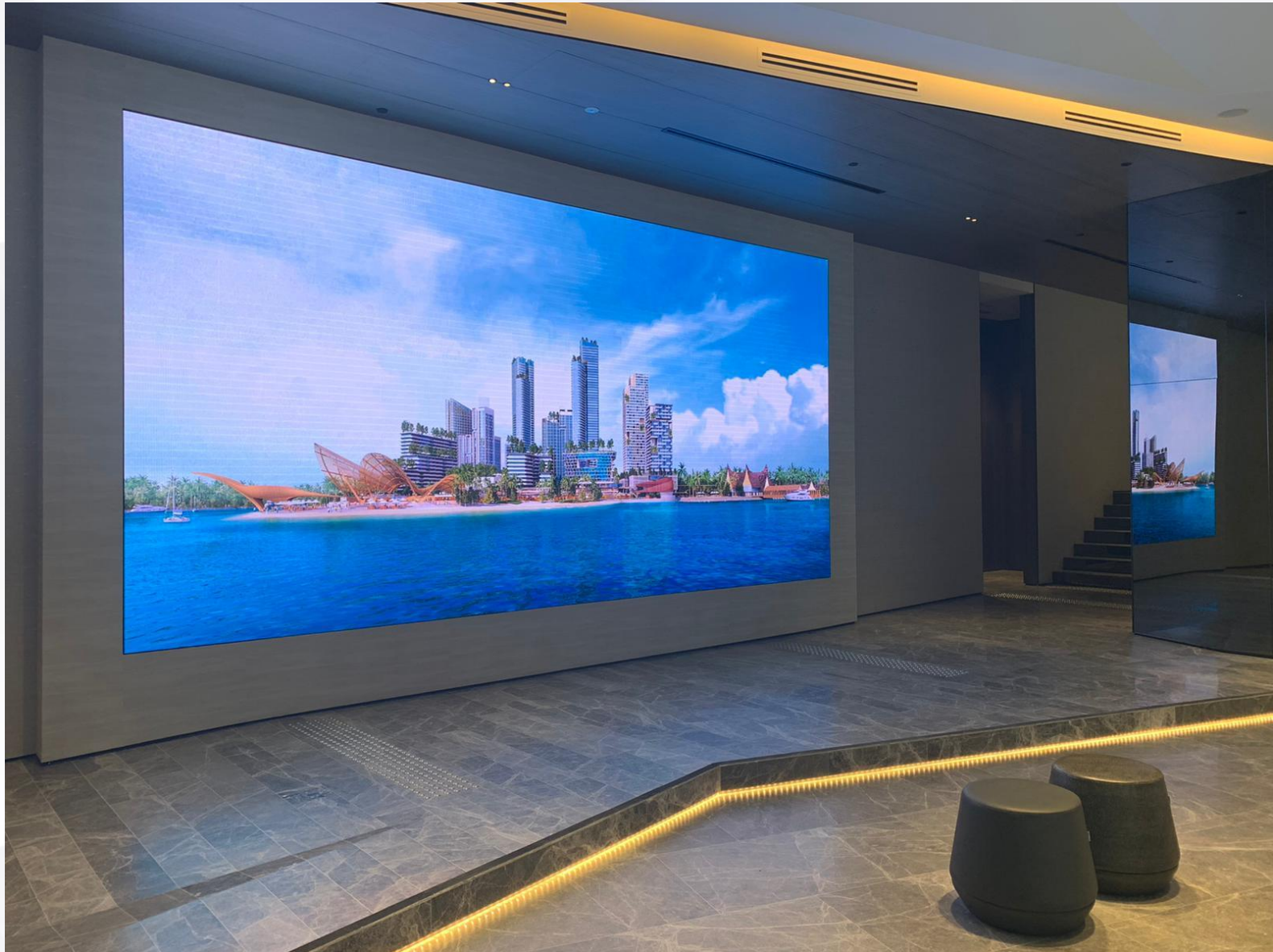
18 Robinsons by Tuan Sing Holdings, 2019 P2.5 Indoor Hard Module (6m x 3m)
